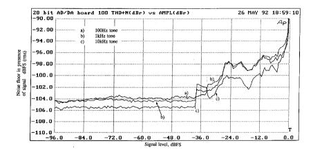
Figure 1 - THD versus level for a leading `20 bit' ADC/DAC codec pair.
