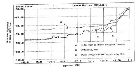
Figure 2 - THD versus level for another ADC/DAC pair, showing the effect of limiting the wordwidth to 16 bits, with and without `dynamic range enhancement'.
