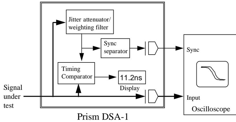
Figure 1 - Weighted interface jitter measurement
