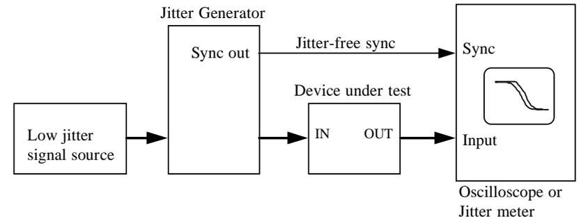
Figure 3 Jitter tolerance and transfer function measurement
