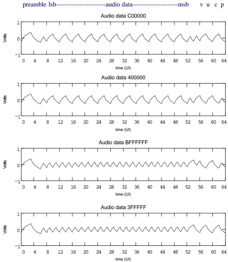
Simulated output after transmission through a 100m length of cable with capacitance 150pF/m and resistance 90ohms/km
