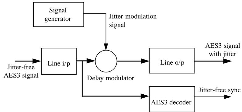
Figure 2 - Jitter modulator block diagram
